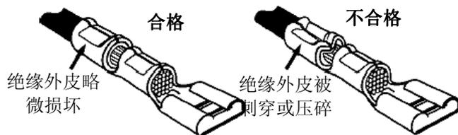
■ 支撑绝缘外皮的压接
